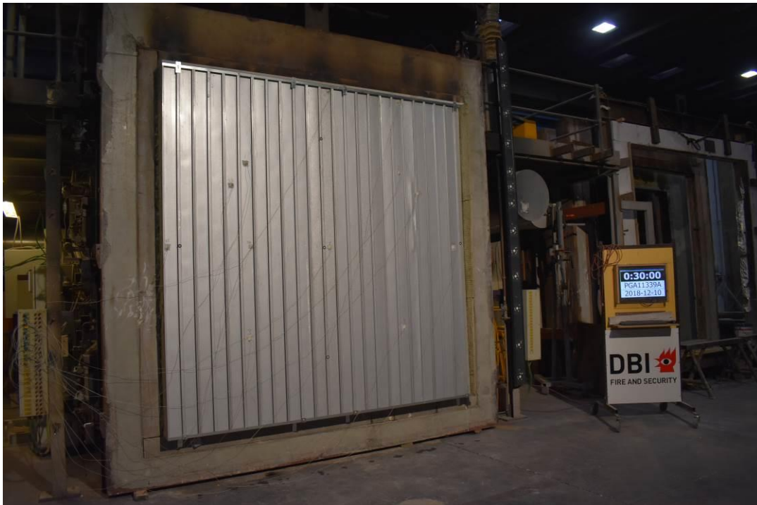
Photo No. 12 The test specimen seen from unexposed side after 30 minutes of testing
