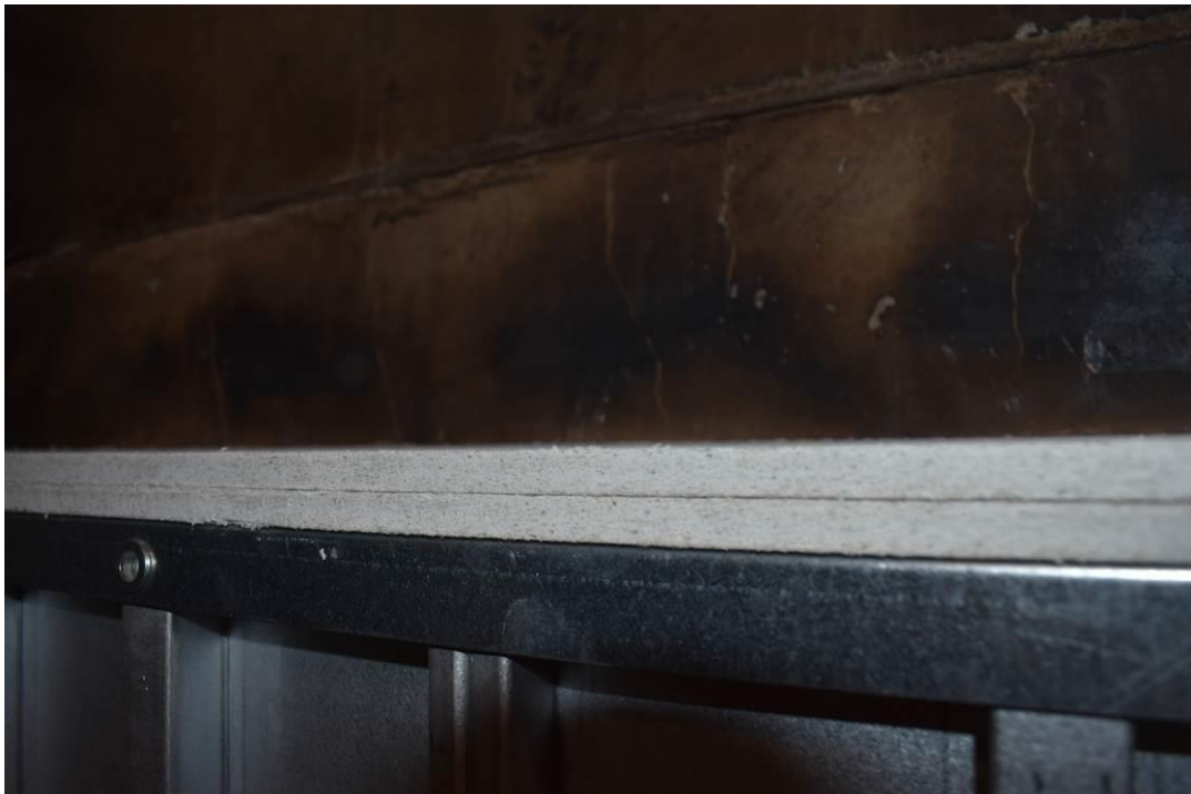
Photo No. 6 The test specimen seen from unexposed side at upper edge – packed with non-combustible boards
