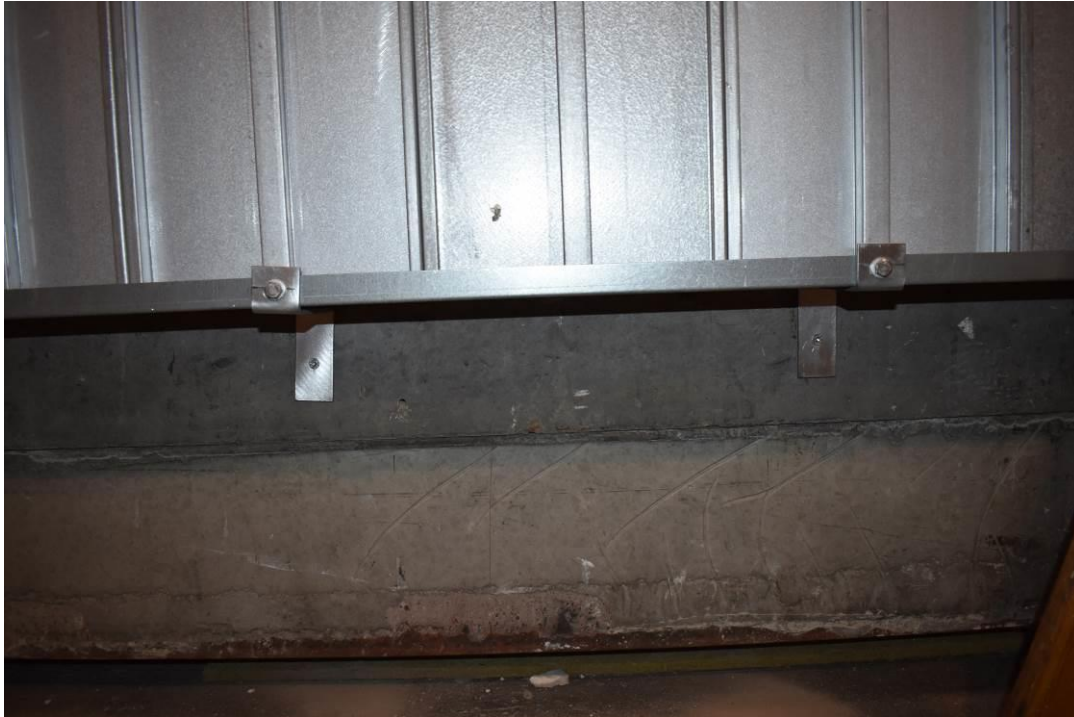
Photo No. 5 The test specimen seen from unexposed side at lower edge – attached to the concrete frame with Z-profiles
