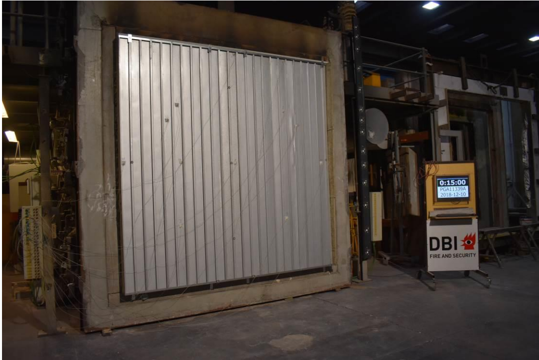
Photo No. 11 The test specimen seen from unexposed side after 15 minutes of testing
