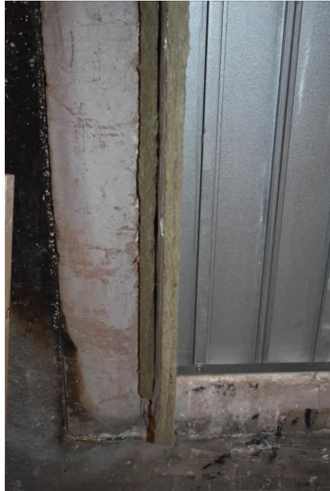
Photo No. 3 The test specimen seen from exposed side at free edge – packed with stone wool
