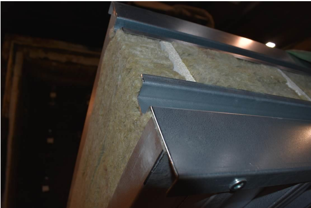
Photo No. 2 Upper edge of test specimen – edge profile of galvanized steel, seen at free edge
