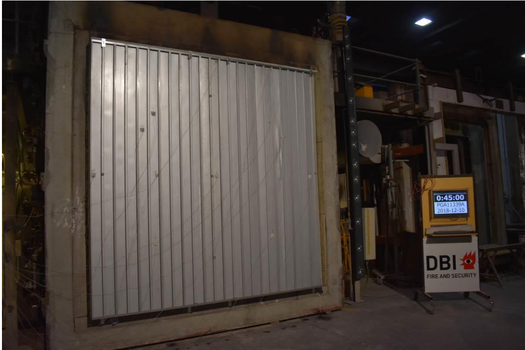
Photo No. 13 The test specimen seen from unexposed side after 45 minutes of testing
