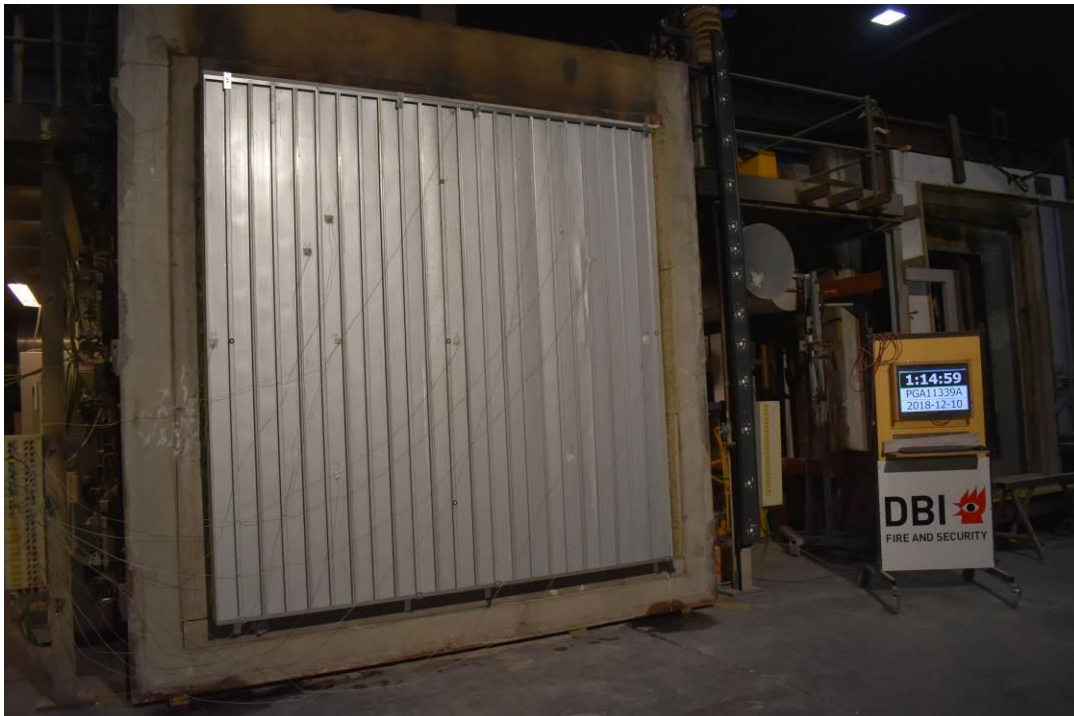
Photo No. 16 The test specimen seen from unexposed side after 75 minutes of testing
