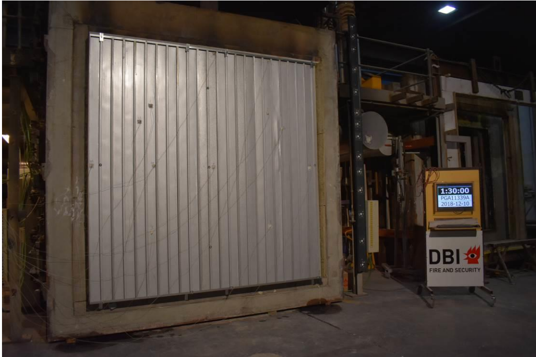
Photo No. 17 The test specimen seen from unexposed side after 90 minutes of testing
