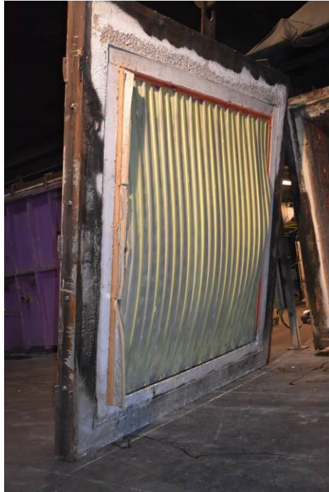
Photo No. 19 The test specimen seen from exposed side after testing
