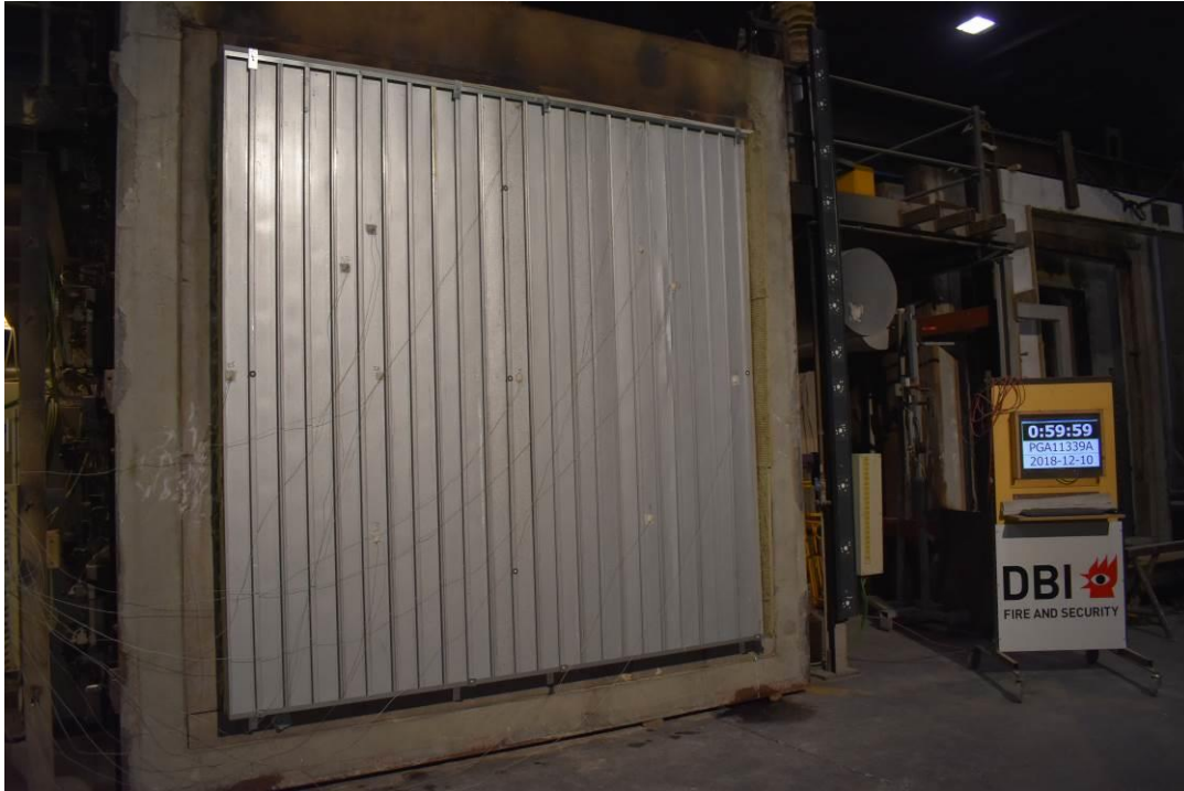
Photo No. 15 The test specimen seen from unexposed side after 60 minutes of testing
