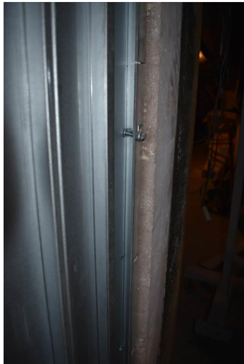
Photo No. 8 The test specimen seen from exposed side at fixed edge – attached to the concrete frame via steel profile
