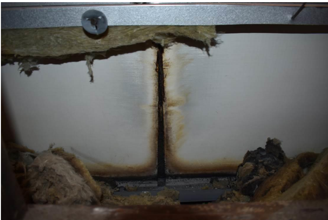
Photo No. 14 The glued joint in a M4 composite board after testing
