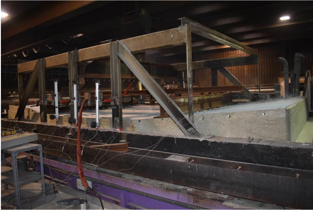
Photo No. 11 The unexposed side after 30 minutes of testing
