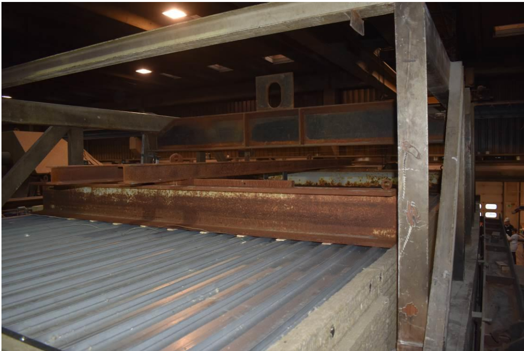
Photo No. 8 The unexposed side of the test specimen at testing start
