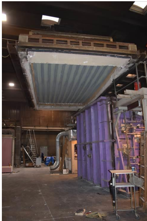
Photo No. 12 The exposed side of the test specimen after testing
