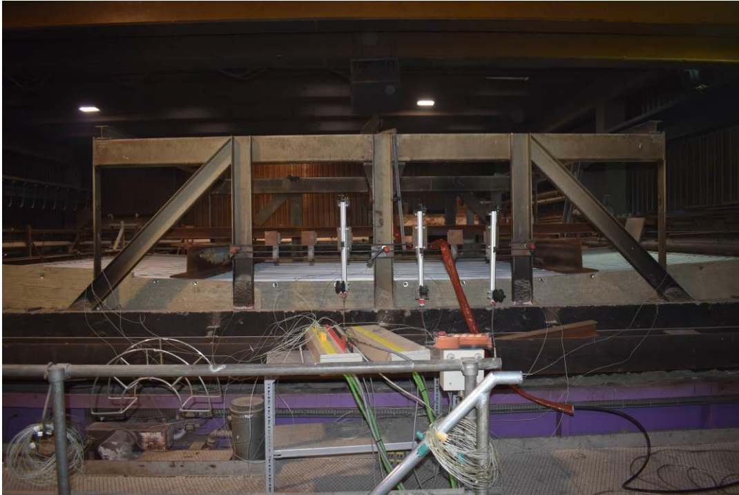
Photo No. 9 The unexposed side of the test specimen after 15 minutes of testing
