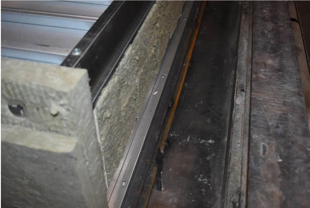
Photo No. 5 The test specimen simple supported in the test frame before testing
