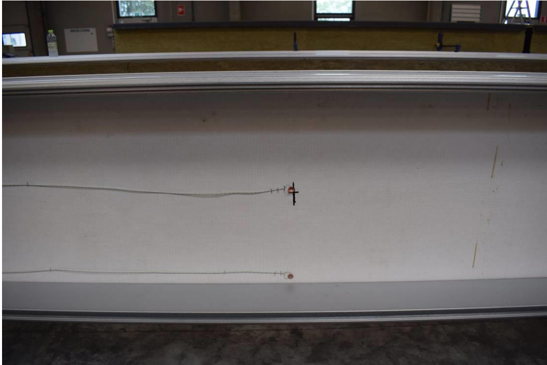
Photo No. 3 The internal thermocouples mounted on the M4 composite boards
