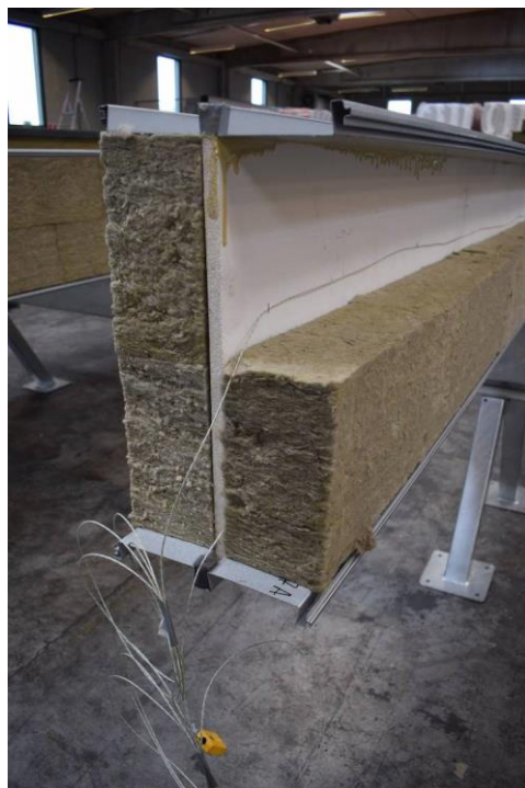
Photo No. 4 The set-up of an individual insulated beam at the sponsors location
