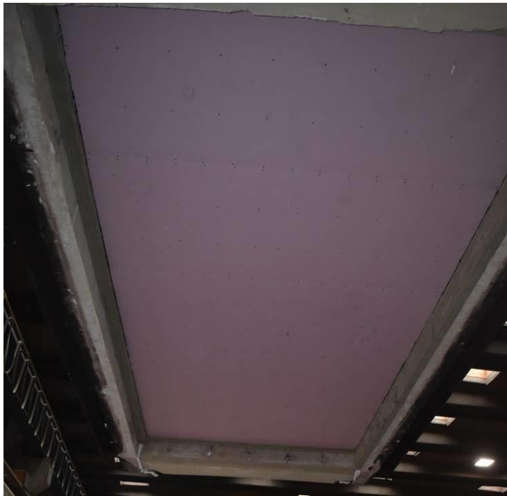
Photo No. 14 The test specimen seen from exposed side before testing
