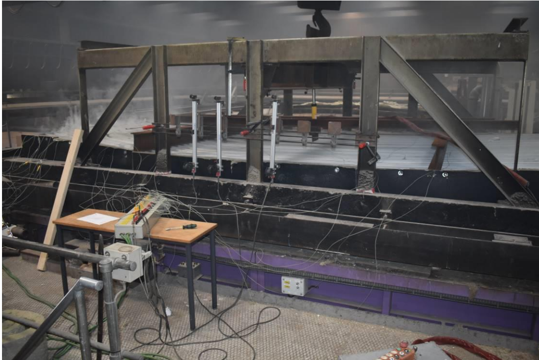
Photo No. 17 The test specimen seen from unexposed side after 87 minutes of testing
