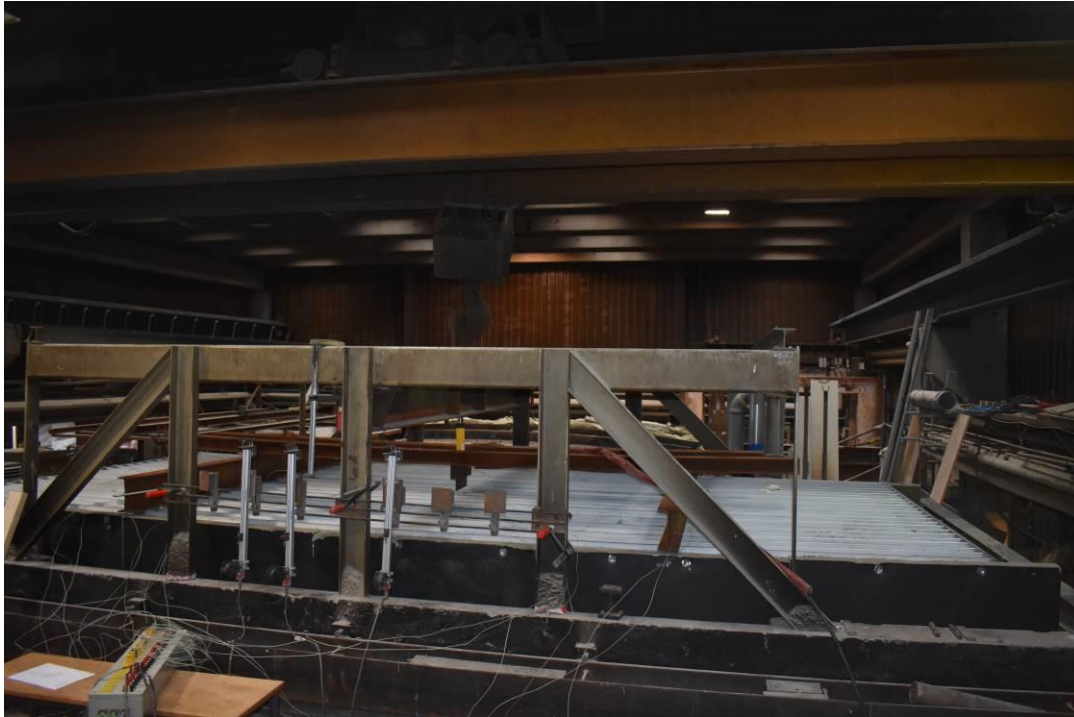
Photo No. 15 The test specimen seen from unexposed side at testing start
