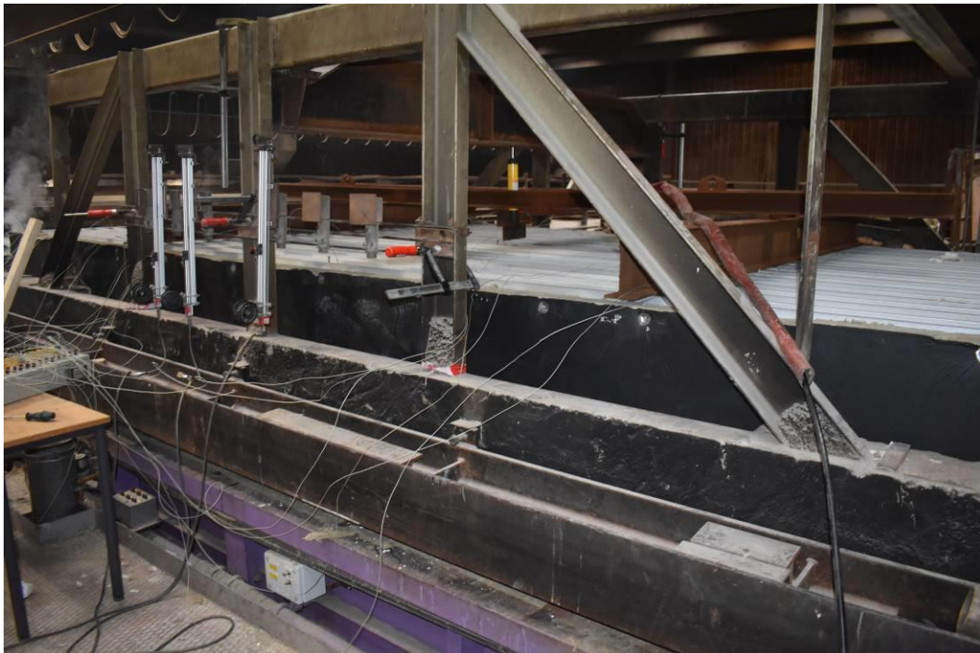
Photo No. 16 The test specimen seen from unexposed side after 38 minutes of testing
