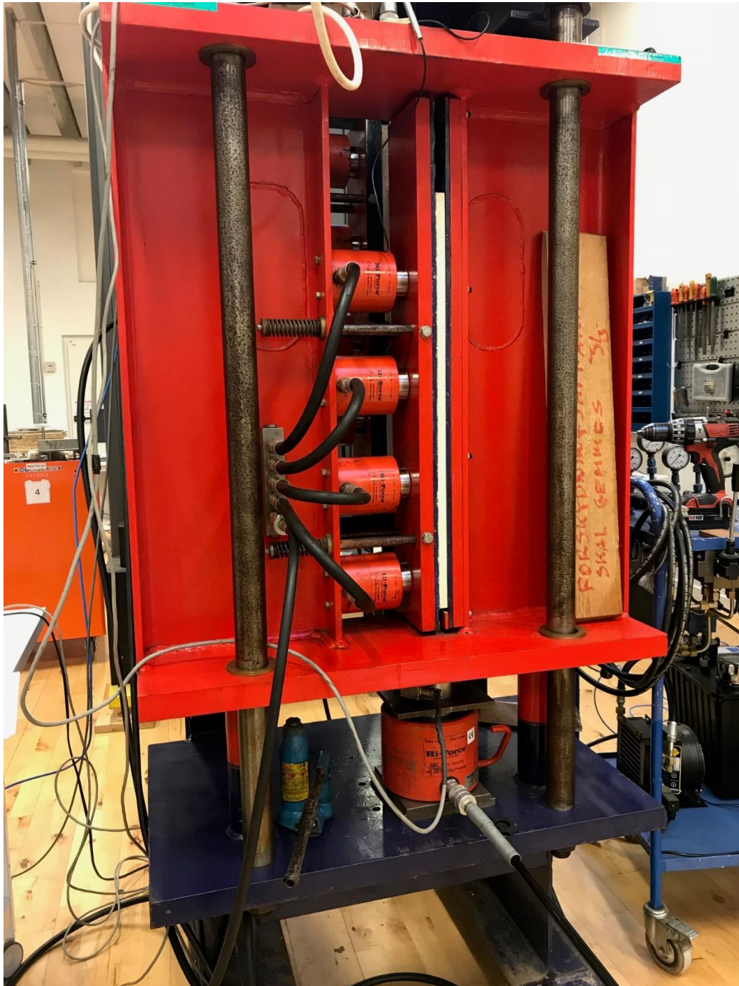
Test specimen in test apparatus. Hydraulic grips with steel floor plates and four hydraulic cylinders. One hydraulic cylinder for the application of load via an electronic load cell.
