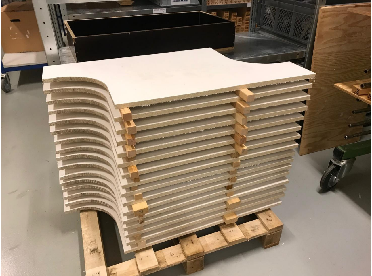
Test specimens cut for testing of panel shear according to EN 789.
