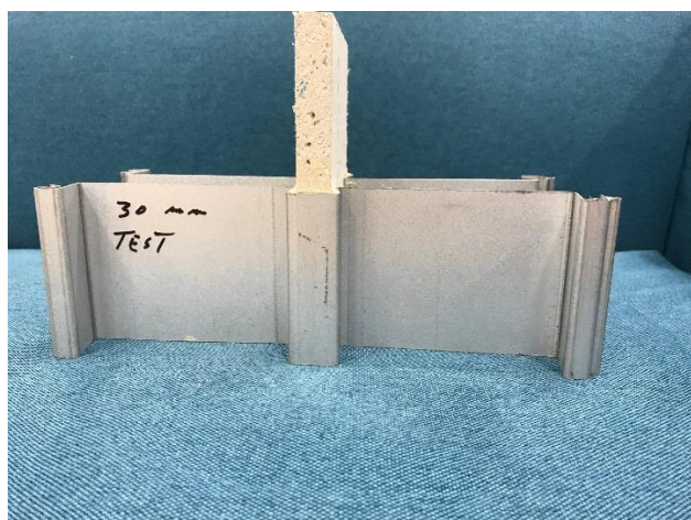
Test specimens – glue line length 20, 30 or 40 mm
